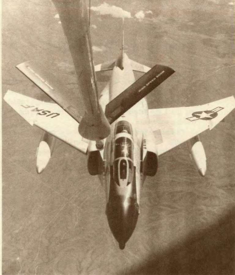
Approaching precontact position, trim for the tanker's downwash and stabilize. Hold until cleared by the boomer. Look under canopy bow to view director lights after you make contact, then just fly good, smooth, formation.
